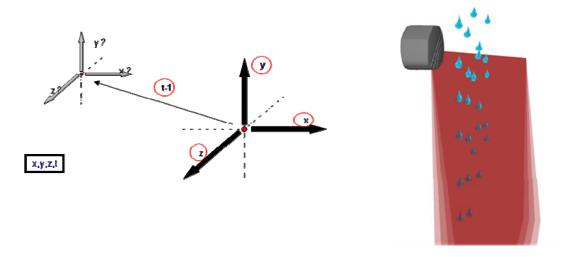
A third information is the ability to remember the state of the previous scan and verify if the situation "t" is equivalent to the situation "t-1". A small object (like rain, snow,...) that crosses the area will therefore also be filtered.
