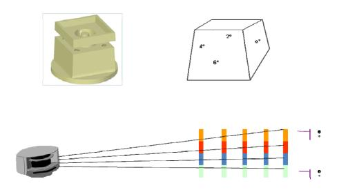
This gives a certain "weight" to the detected object. Indeed it is possible to differentiate between an object, like a raindrop, that will be seen in an instant 't' only on one of the four planes and a larger object that will affect all levels. The limitations of this weight will obviously depend on the application and are set through the detection algorithms.
